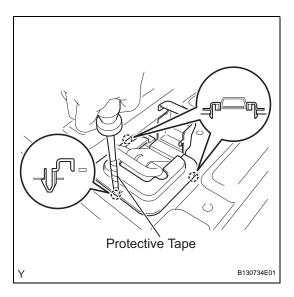
(b) Using a screwdriver with its tip wrapped in protective tape, disengage the 3 claws and remove the tether anchor cover.
